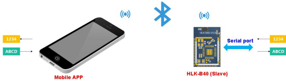
Figure 4 One-to-one Bluetooth connection transmission function schematic
